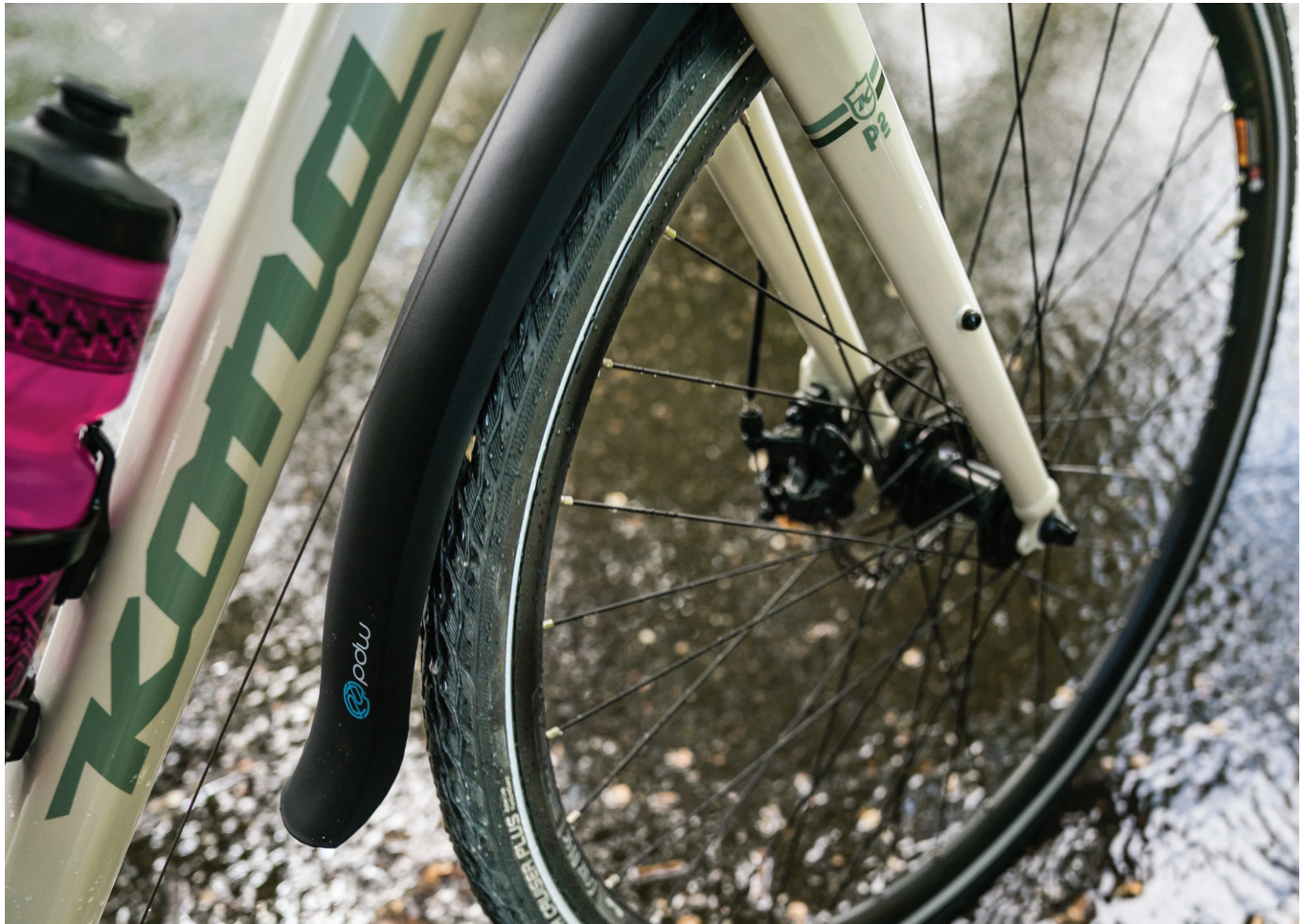
Figure 4: Sodapop front fender configuration
